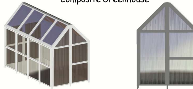
Figure 5: 3D views of the greenhouse structure design
