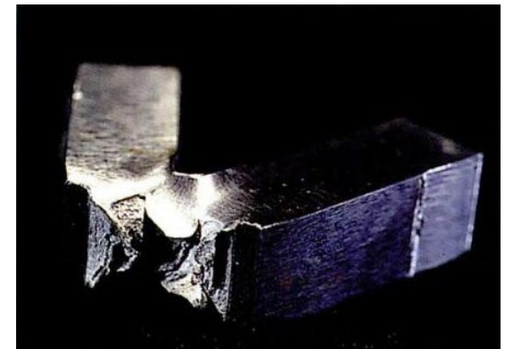
Modern high quality steel - Ductile fracture
