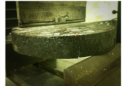
asphalt specimen subjected to pure mode III
