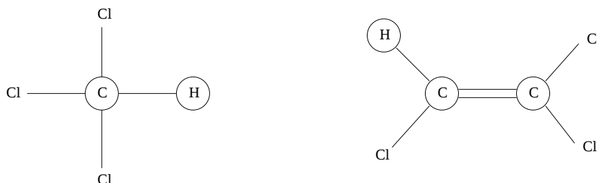
Figure 17.1 Chloroform (left) and trichloroethylene (right) molecules. The hydrogen ^1H , carbon ^{13}C , and fluorine ^{19}F atoms whose spin-1/2 nuclei serve as qubits are circled. The chlorine nuclei have zero spin and are not qubits.
