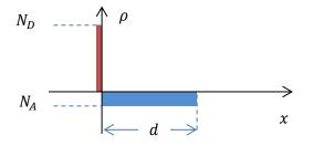
In the p-doped layer, we assume that the depletion zone extends over a width d that is less than the film thickness. Throughout this depleted region, we may assume a negative charge density equal to the acceptor concentration  $N_A$ . Since the ITO is highly doped, its depletion zone is very narrow and can be treated like a surface charge. The result is a one-sided p-n junction, similar to a Schottky-junction.
