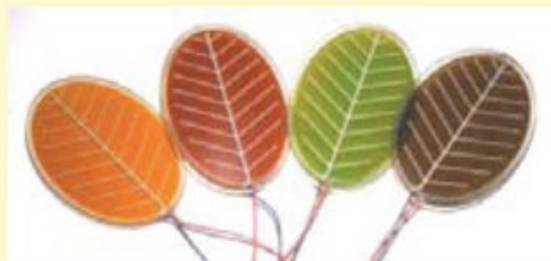
Leaf-shaped transparent DSC with four colors
