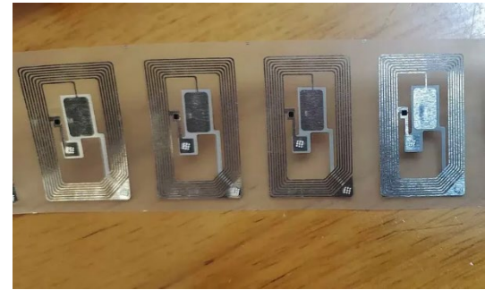
Plastic 12-bit RFID Tag and Read-out System with Screen-Printed Antenna
