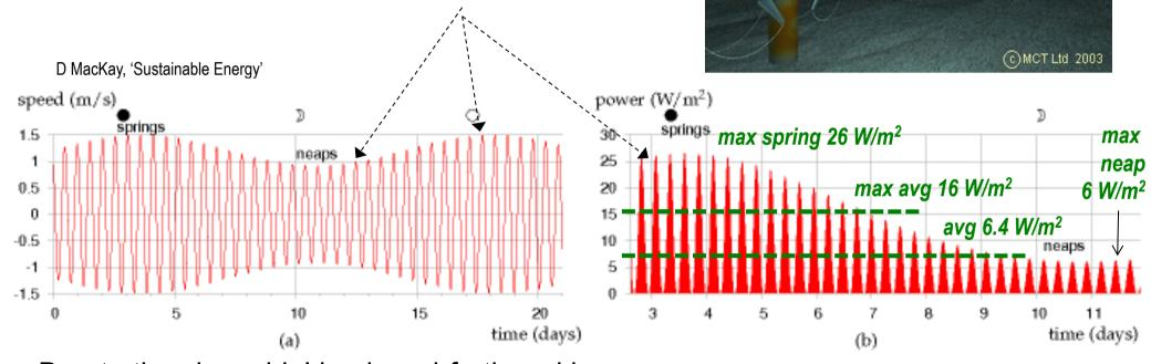
Due to the sinusoidal back-and-forth rocking of tides every 6h, the average effective current is ≈ 0.4•peak current.
