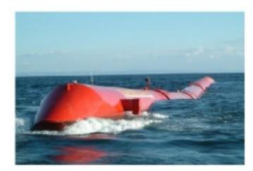
1 km<sup>2</sup> area = 400 m long x **2.5 km wide incoming wave**, 3 rows of 40 Pelamis (120 Pelamis). Assume **30 kW / m** waves ( $c_0 = 12.5 \text{ m/s}$ ,  $y_0 = 1 \text{ m}$ )  $\rightarrow$  2.5 km wide equals 75 MW<sub>e</sub> 1 every 60 m in each row, 1 every 20 m in the wave front, staggered from row 1 to row 3
