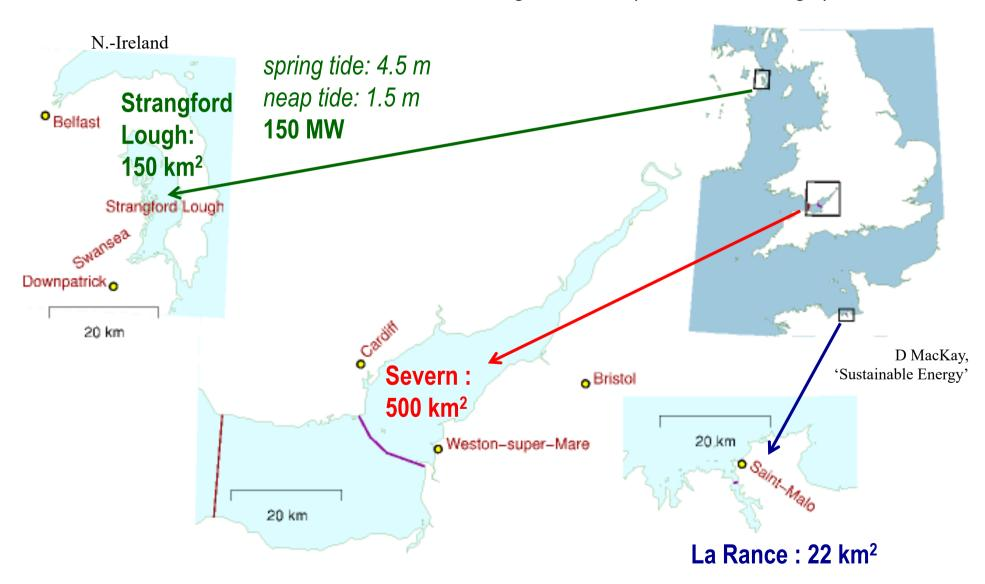
spring tide: 11  $m \Rightarrow max 14.3 \text{ GW}_e$ neap tide: 6  $m \Rightarrow max 3.9 \text{ GW}_e$
