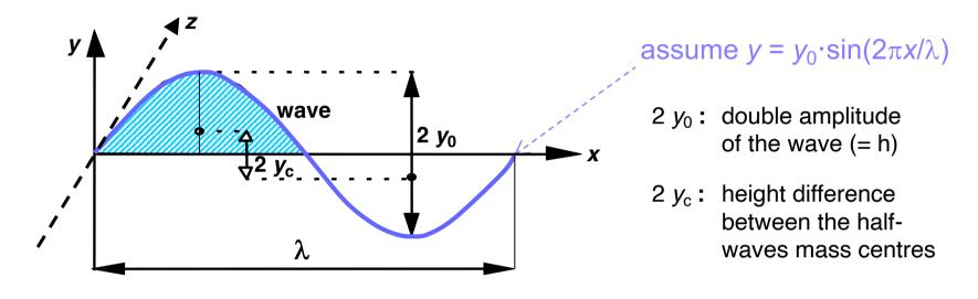
Mass  $M_z$  per unit length of the wave front in z-direction (kg/m):
