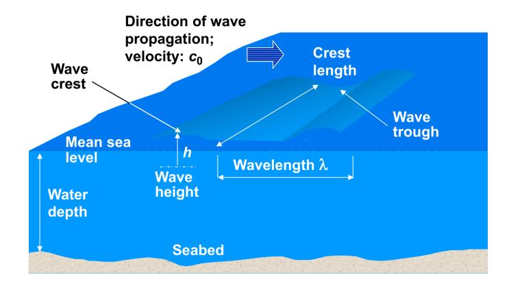
The energy that can be extracted from a wave corresponds roughly to the potential energy **liberated by the collapse of the wave** crest, i.e. the energy obtained when the mass M of the "half-wave" falls from a height 2  $y_c$ , where  $y_c$  represents the mass centre of the "half-wave".
