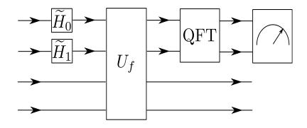
The circuit is initialized with the state  $|\psi_0\rangle = |0\rangle \otimes |0\rangle \otimes |0\rangle \otimes |0\rangle$ . We will denote  $|0\rangle \otimes |0\rangle = |0\rangle$ ;  $|0\rangle \otimes |1\rangle = |1\rangle$ ;  $|1\rangle \otimes |0\rangle = |2\rangle$ ;  $|1\rangle \otimes |1\rangle = |3\rangle$  and define for  $x, y \in \mathbb{Z}$ :
