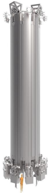
Central solenoid \text{Nb}_3\text{Sn} , 13T
