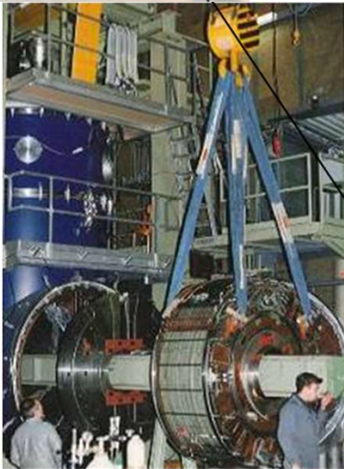
Magnet and sample cooled by forced flow of supercritical He (4.5 K- 20 K)
