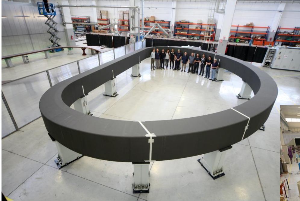
Toroidal Field coils winding pack in ASG – La Spezia
