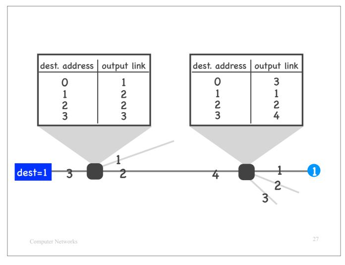
Each end-system has an address, which is called IP address (as we have already seen in previous lectures). Let's say our destination has IP address #1 (which is not really a valid IP address, but we will pretend it is, to keep the picture simple).
