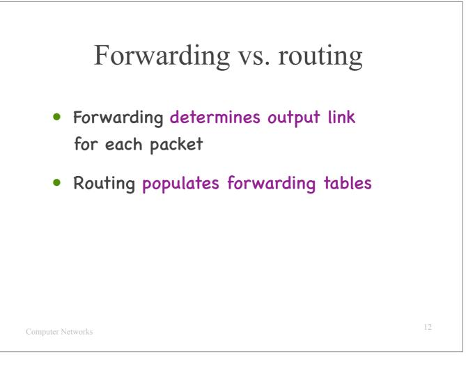
To conclude this first part, a network layer provides at least two basic functions: forwarding and routing. Forwarding relies on forwarding tables, while routing populate the forwarding tables that are needed for forwarding.
