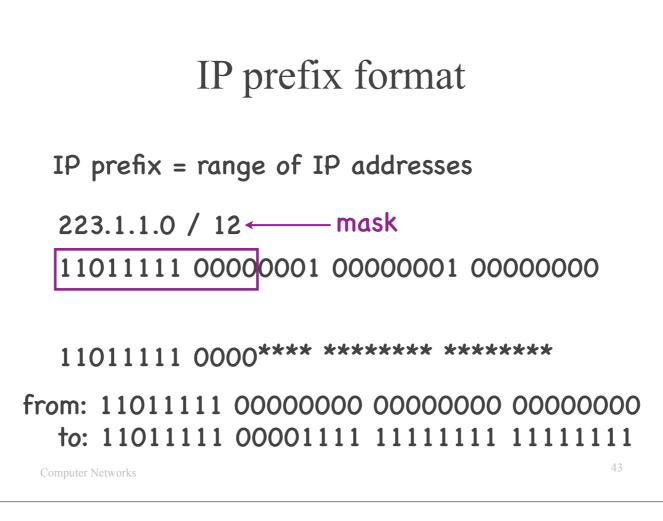
When the mask is not a multiple of 8, it's a bit harder to visually determine the range of IP addresses covered by an IP prefix. Please don't try it! It's better to be conservative and follow the right steps: write the entire prefix in binary form and identify the smallest and largest IP address that it covers.
