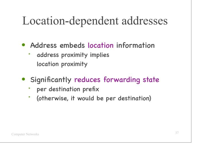
So: IP addresses are location-dependent, meaning that an IP address embeds location information, and address proximity typically implies location proximity.
