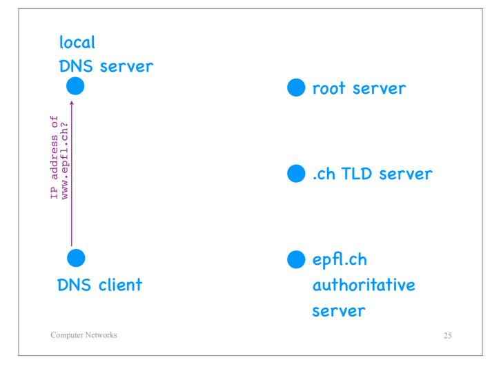
The way I have described things, when a DNS client makes a request, it has to wait until 4 different DNS servers are contacted, and this may take a long time.
