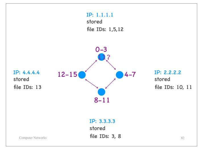
Suppose this is a P2P system that consists of 4 peers, which have these IP addresses.
