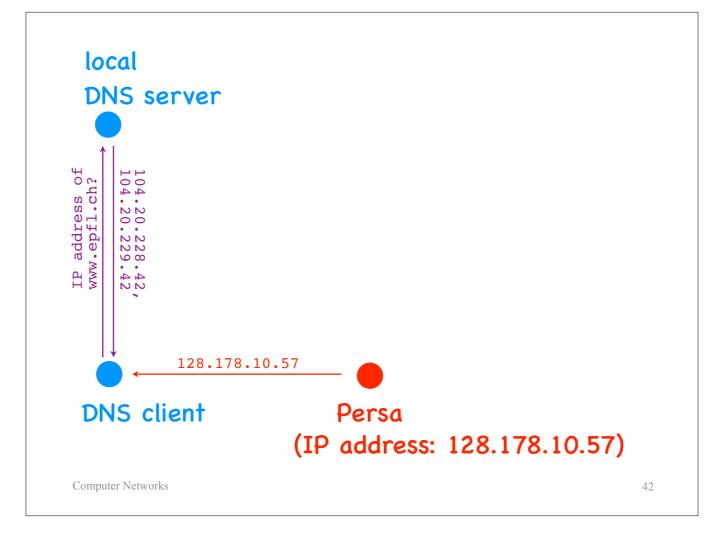
Suppose we have a DNS client, which asks its local DNS server for the IP address of www.epfl.ch.
