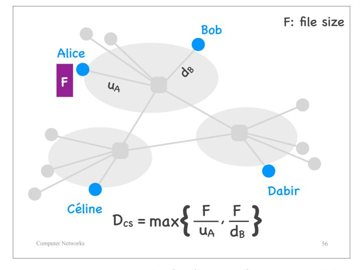
So, in general, the file distribution time is equal to the transmission delay of the file over the first or the second link, whichever one is bigger.
