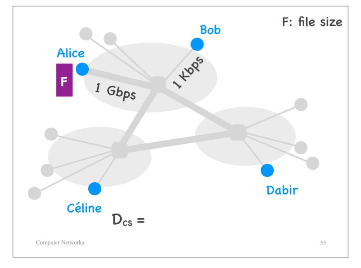
If the link with the smallest transmission rate is the second link, then the file distribution time is the transmission delay of the file over the second link plus some other components that we can ignore.
