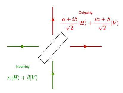
5) The semi-transparent mirror leaves photons in state  $S(\alpha | H \rangle + \beta | V \rangle$ ). The state is then measured by the detector D which detects photons in state  $|V\rangle$ . Therefore, the probability of finding a photon in D is the probability of finding a photon in state  $|V\rangle$  given that
