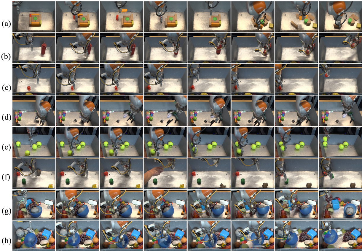
Fig. 4. Eight grasps from the QT-Opt policy, illustrating some of the strategies discovered by our method: (a), (b) pregrasp manipulation; (c), (d) grasp readjustment; (e), (f) grasping dynamic objects and recovery from perturbations; and (g), (h) grasping in clutter.
