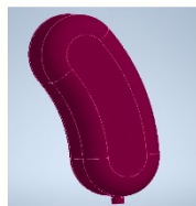
Fig. 1: Pressurized ergonomic portable compressed air tank
