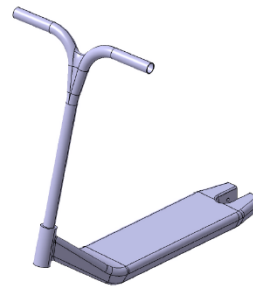
Rental Electric Scooter - Flax fibers deck & steering pole
