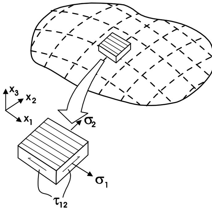
$$[S_{ij}] = \begin{bmatrix} S_{11} & S_{12} & 0 \\ S_{12} & S_{22} & 0 \\ 0 & 0 & S_{66} \end{bmatrix} = \begin{bmatrix} 1/E_1 & -\nu_{21}/E_2 & 0 \\ -\nu_{12}/E_1 & 1/E_2 & 0 \\ 0 & 0 & 1/G_{12} \end{bmatrix}$$
