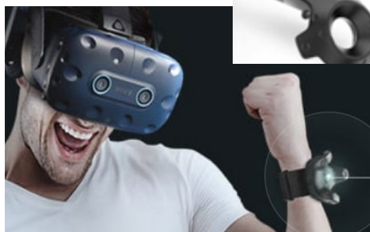
HTV-Vive basestation and sensors on HMD, tracker & controllers
