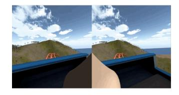
Note the virtual nose serving as a rest frame in a concept demo from Purdue University + [WWSOI18]
