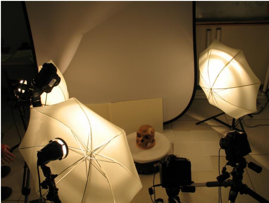
Multi-view reconstruction setup
