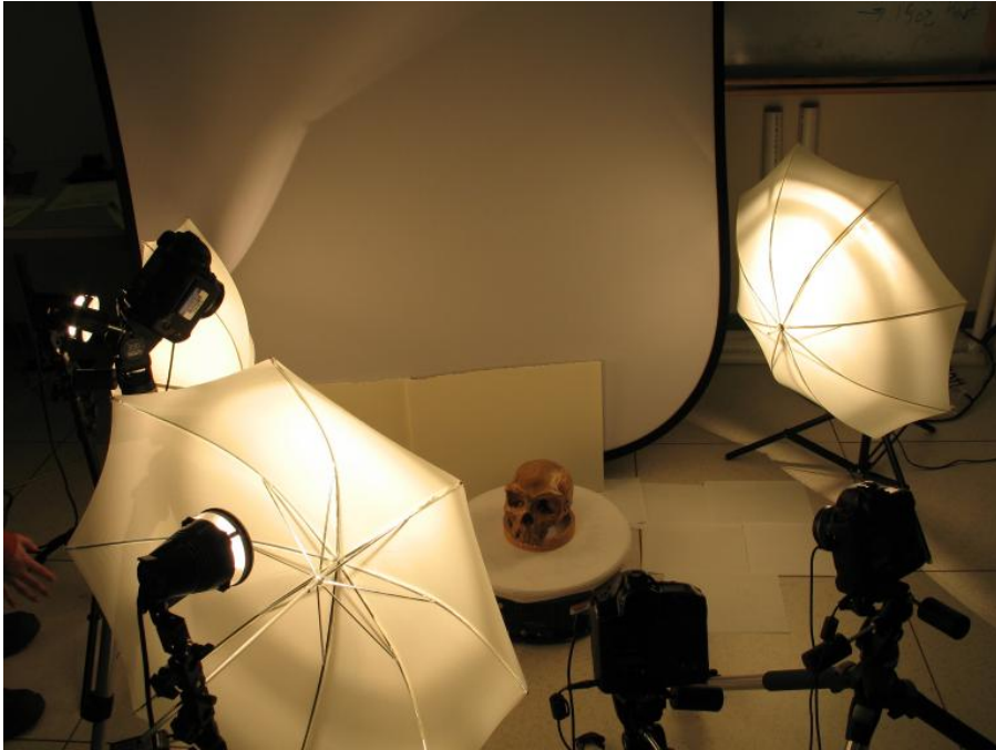
Multi-view reconstruction setup
