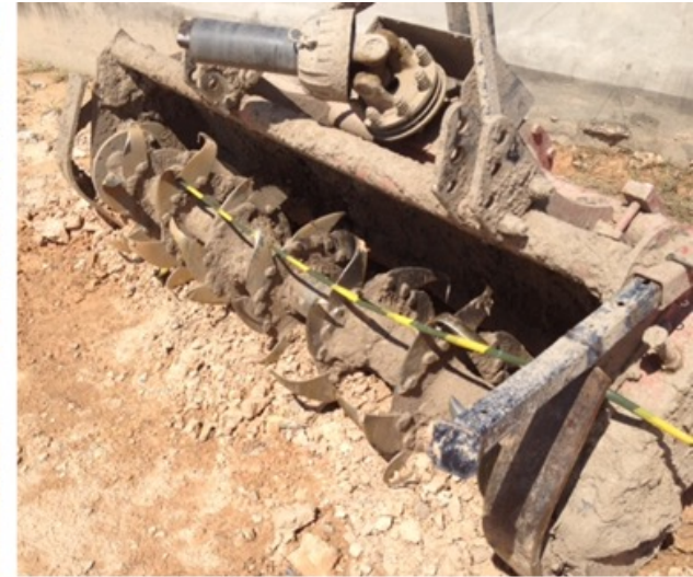
Rotavator: Effective at mixing soils and crumbling soils from depths of <15 cm
