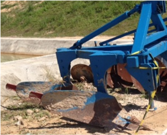
Moldboard Plow: Effective at breaking lumps and turning over soil from depths of 30 cm
