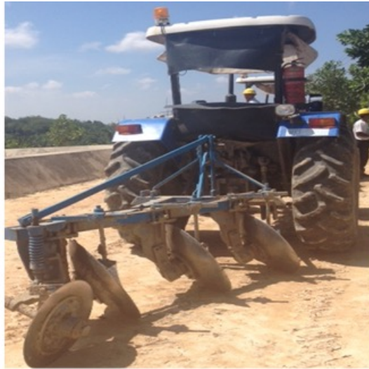
Disc Plow: Effective at loosening, turning over soil from depths of 30 cm
