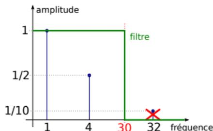
$$\text{Spectre } \hat{X} = \text{Spectre } X \times \text{filtre}$$
