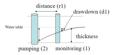
$$Q = \frac{1.366K(h_2^2 - h_1^2)}{\log\left(\frac{r_2}{r_1}\right)}$$
